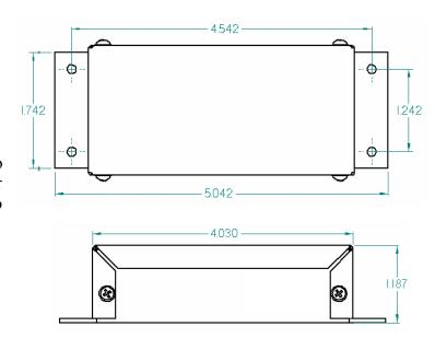
When the desired location is selected, secure the heater controller via the 4 mounting holes. Route the wiring between the probe, controller, panel, and power source, as described below.
